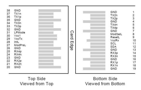
Figure 2. Electrical Pin-out Details
