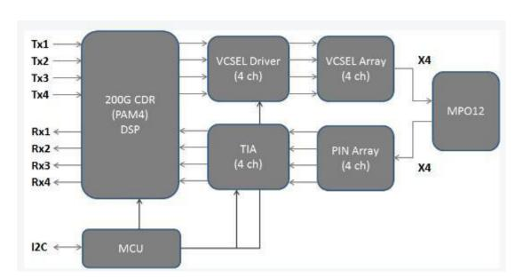
Figure 1. Module Block Diagram
