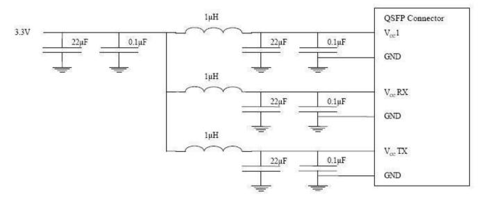
Figure 3. Host Board Power Supply Filtering
